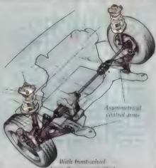
With front-wheel drive, the engine is offset to the right. To counteract this imbalance and permit equal response in left and right turns, the 626 uses unique asymmetrical control arms (the right arm is 1.4 inches shorter than the left).
